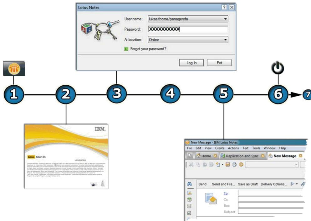
1. The IBM Notes Client is launched and the local MarvelClient binary (for example "mc.dll" or "pmc.dll" on Windows) is invoked by the IBM Notes client as an Extension Manager ("EXTMGR\_ADDINS" parameter in notes.ini)
